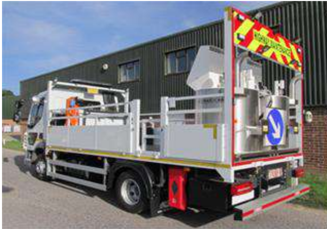
10 Tonne Screed Truck
